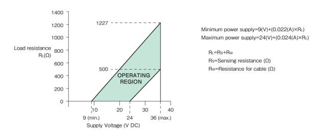
When the load resistance 500  $\Omega$  or more are needed, 24V DC supply voltage or more is necessary.
