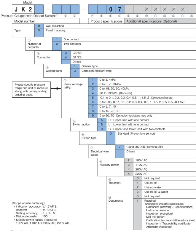
OAs setting scale on dial includes setting error, ensure the use of master gauge and reference pressure gauge to maintain accurate setting.
