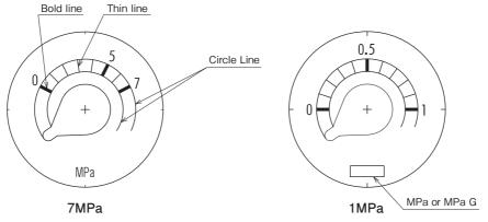
Note: The range of the scale at different angles.
