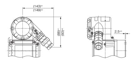
[\*1] Size: Flameproof cable gland, Connection 3/4 [\*2]Size: Flameproof cable gland, Connection G1/2 [\*3] Size: Bracket size
