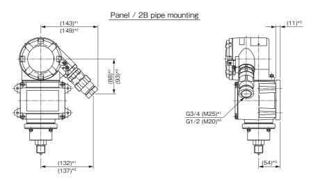
[\*1] Size: Flameproof cable gland, Connection 3/4 [\*2]Size: Flameproof cable gland, Connection G1/2 [\*3] Size: CD75 Compatible bracket (Optional)
