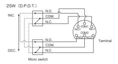
\*Please connect the (+) polarity with common terminal COM1 for S.P.D.T. specification for 1 point of contact direct current.
